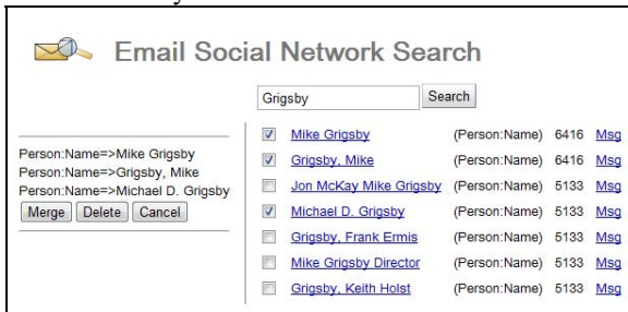
Figure 5. Prototype GUI with results of full-text search and several objects (aliases) selected for possible merge or delete. When these object aliases are merged, subsequent search returns better results for any of them.
